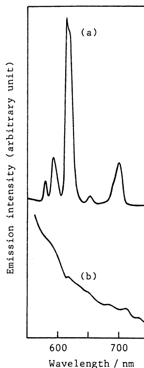
Fig. 10. Fluorescence spectra of mononuclear Eu(III) (a) and dinuclear V^{IV}O -Eu(III) (b) complexes in solid state. Exciting wavelength is 394 nm. Slit widths (nm) of (excitation and emission sides) are (2 and 2) for (a) and (10 and 5) for (b). Ordinate scale is \times 64 .
