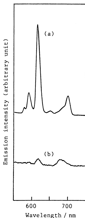
Fig. 8. Fluorescence spectra of mononuclear Eu(III) (a) and dinuclear V^{IV}O -Eu(III) (b) complexes in DMF. Concentration of complex is 5 \times 10^{-3} mol dm^{-3} . Exciting wavelength is 342 nm. Slit widths (nm) of (excitation and emission sides) are (10 and 5). Ordinate scales are \times 512 for (a) and \times 1024 for (b).
